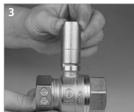
Install the cylindrical extension placing it on the ball valve rod and paying attention to the opening direction
