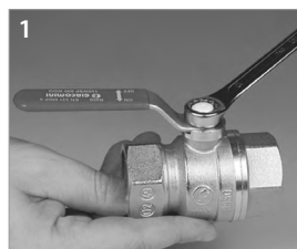
Loosen the nut with the proper wrench
