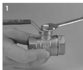
Remove the nut with the proper wrench
