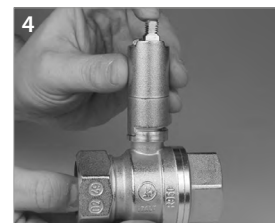
Screw the extension central pin on the ball valve rod and tighten completely using the ball valve lever
