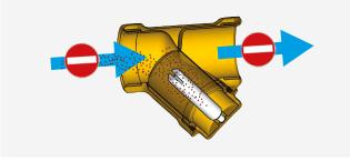
**2)** Unscrew the cap and remove the magnet and the metal mesh mounted on it.
