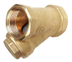
R74M si a magnetic Y-filter, inspectable, suitable for the distribution of non-hazardous fluids (group 2, according to the PED Directive) which are safe for use with copper alloys. The filter features a metallic mesh and a magnet, which was designed to prevent solid impurities from entering into the piping and, by depositing residues, reducing the width of the passage, thus increasing losses of pressure and oxidation.
