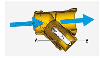
The flow enters the filter and is slowed down, allowing for the separation of the solid impurities present in the fluid. The solid impurities are separated when they collide with the metal mesh (A) and ferrous particles are retained by the attraction force generated by the magnet (B).
