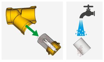
**4)** Replace the magnet and the metal mesh on the cap and screw it on the filter body.
